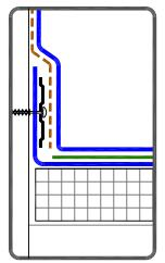
OPTIONAL: SEAM PLATE/FASTENER MAY BE INSTALLED INTO THE STRUCTURAL DECK UP TO 6" (15cm) FROM ANGLE CHANGE.
