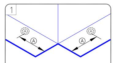
FASTEN MEMBRANE AND FLASH CURB OR WALL WITH CURED EPDM MEMBRANE FOLLOWING STANDARD PROCEDURES USING BONDING ADHESIVE and PAS SEAM TAPE.
