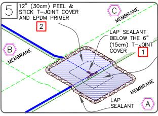
APPLY 6" (15cm) PEEL & STICK T-JOINT COVER AND 12" (30cm) PEEL & STICK T-JOINT COVER OR PEEL & STICK UNCURED EPDM CENTERED OVER THE INTERSECTING POINT OF THE LEADING EDGES OF THE FIELD SPLICE INTERSECTION AS SHOWN.
