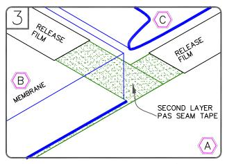
SPLICE SHEET B TO SHEET A AND APPLY SECOND PIECE OF PAS SEAM TAPE BETWEEN SHEET B AND C. TRIM RELEASE FILM AS SHOWN.
