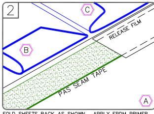
FOLD SHEETS BACK AS SHOWN. APPLY EPDM PRIMER TO THE SPLICE AREA ON BOTH SURFACES AND ALLOW TO FLASH-OFF. APPLY PAS SEAM TAPE WITH RELEASE FILM ALIGNED WITH MARKED LINE.
